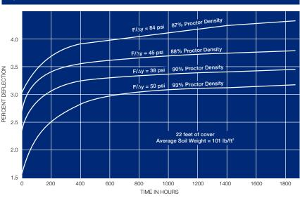
Deflection as a function of time for PVC pipe buried in an embankment. Source: Utah State University
