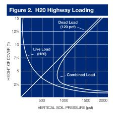
shows the effect of H20 live loads at various depths of cover. From this chart you see that highway live loads are not significant at depths of 4 feet or greater. Live loads are also shown in Table 2.
