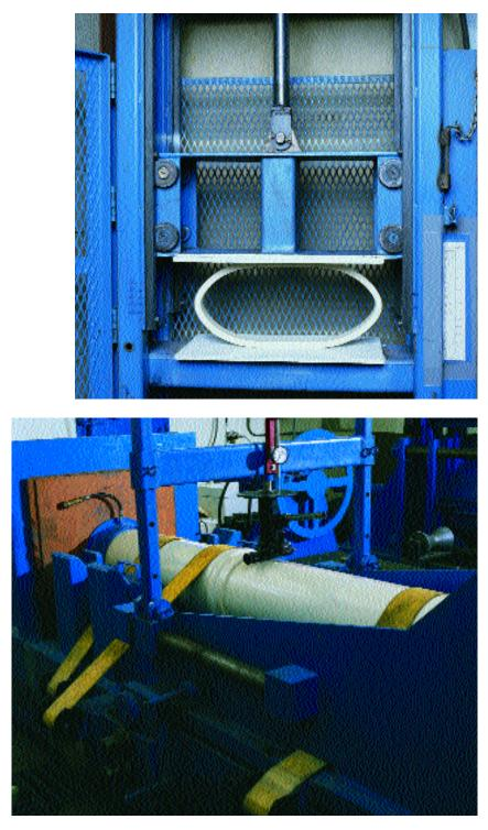
Joints are tested in our laboratory under both pressure and vacuum to assure quality in the gasket and the fit. As required by ASTM, the tests are performed with the pipe joint bent axially and with the spigot end deflected, simulating adverse field conditions. Infiltration is limited to 50 gal/inch diameter/mile/day—or less—in even the wettest conditions.
